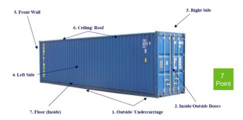
Along with the seven-point inspection process for containers, all tractors and trailers must also be inspected:
